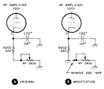
fig. 2. Modifications for the R390A rf amplifier.
